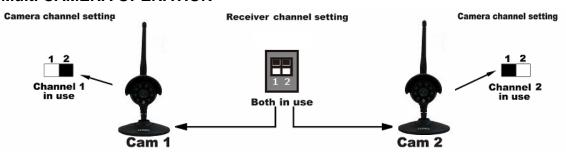
This 900MHz Wireless Color Camera System can support a total of 2 cameras (additional camera is sold separately). When using multiple cameras, set each camera to different channels. The Receiver needs to be set to have 2 cameras switched to ON, to have all attached cameras functioning simultaneously.
